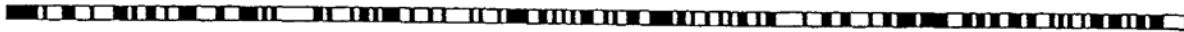
Fig.8. The coded-aperture basic sequence generated by the primitive polynomial h(x) = x^8 + x^6 + x^5 + x^1 + 1 .
